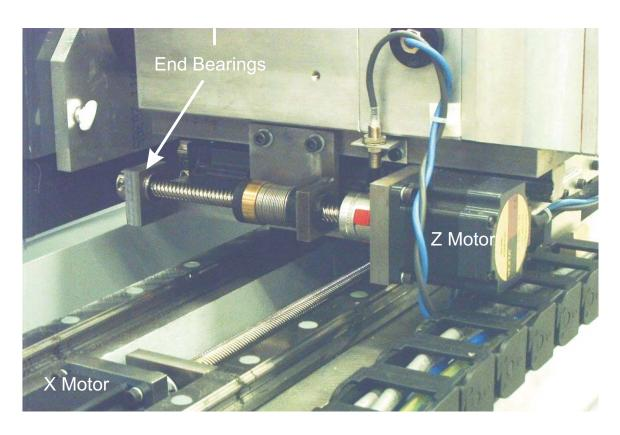
Below is an illustration of the bearing assembly with photos of where they are located on the machine. This is for a three axis machine so you don't have the upper left bearing in the upper left photo.
