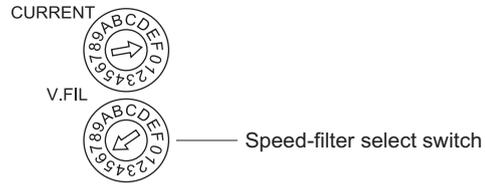
The dial settings and corresponding levels of filter time constants are as follows:
