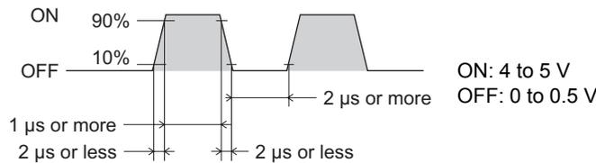
The figure shows the voltage levels of pulse signals.
