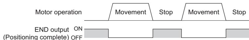
**Note** The timing of the END output turning “ON” after the pulse stops will vary, depending on the conditions of the load, the pulse input, and the speed-filter setting.
