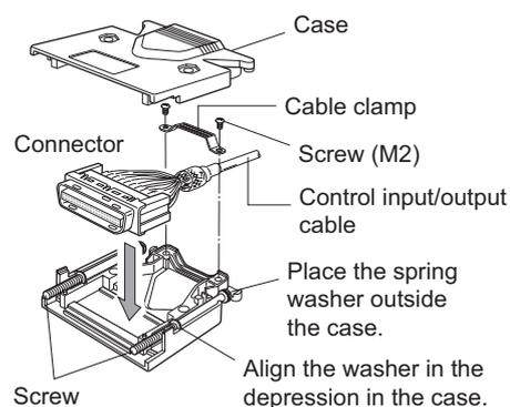
2. Attach the other case and clamp both connector cases together with screws and nuts. Tightening torque: 0.5 to 0.55 N·m (71 to 78 oz-in)
