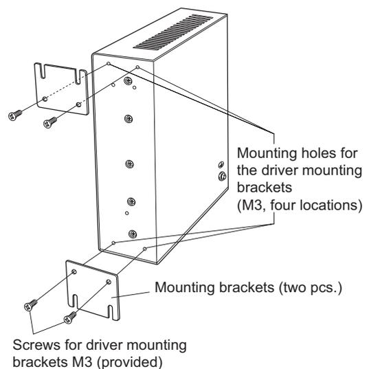
2. Install the driver by securing it with four bolts (M4, not supplied) through the four mounting holes provided. Leave no gap between the driver and plate.
