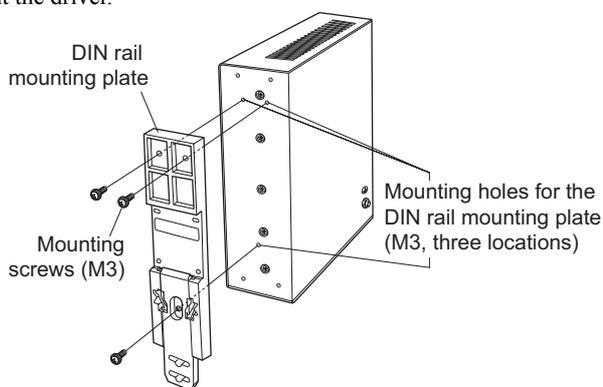
2. Pull the DIN lever down, engage the upper hooks of the DIN rail mounting plate over the DIN rail, and push the DIN lever until it locks in place.
