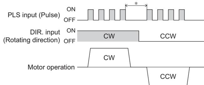
\* The minimum interval time needed for switching the direction of rotation will vary, depending on the operating speed and size of the load. Do not shorten the interval time any more than is necessary.
