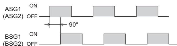
ASG output: Outputs pulse while the motor operates.
