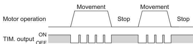
**Note** If TIM. output is to be detected, set the pulse speed at 500 Hz or less. Use the  $\times 10$  input to switch the resolution only when TIM. output is in the “ON” state and the motor stops. If the resolution is switched under any other conditions, TIM. output may not turn “ON” even when the output shaft has rotated  $7.2^\circ$ .
