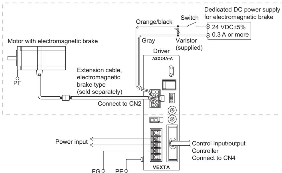
The colors of the two lead wires (orange and gray) extending from the driver's connector side of the flexible extension cable of the electromagnetic brake type differ from those of the extension cable.
