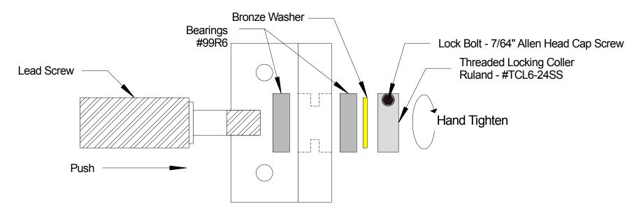
While applying enough pressure to take up any slack, tighten the treaded locking collar ( Hand tighten only! ). Then tighten threaded collar set screw.
