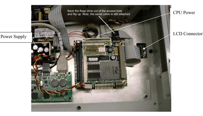
There is also a tall slim board to the left which powers the LCD lamps. The top and bottom connectors have 600v for the lamps (Caution!) and the middle connector is a 12v supply for the LCD controller on the back of the CPU
