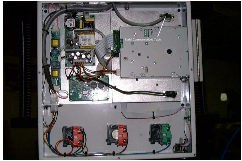
The power supply cable has multiple 5v and ground connections. Typically the 5v is red and ground is black and the third color, yellow or orange, is 12v I would check the power supply voltages and connections (see below) then check the LCD screen connector.
