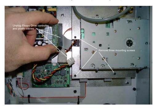
Next, swing the floppy up from the bottom. To do this, you will have to move it left slightly to get it out of the access door hole. (Be care of the CPU power plug in the notch behind the floppy) The serial cable is still attached at this point so you can't remove the floppy drive.
