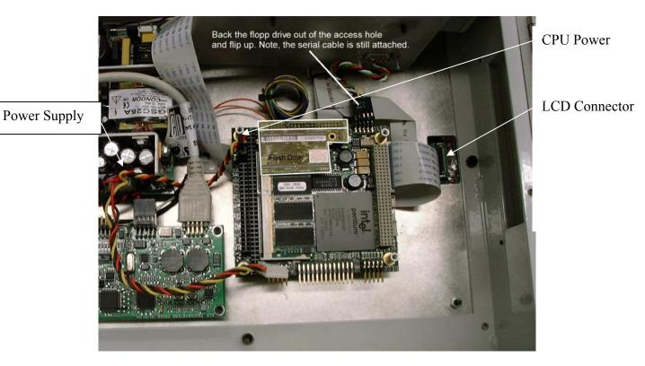
You can check the soldered connection on the short serial cable and make sure it hasn't come unplugged.
